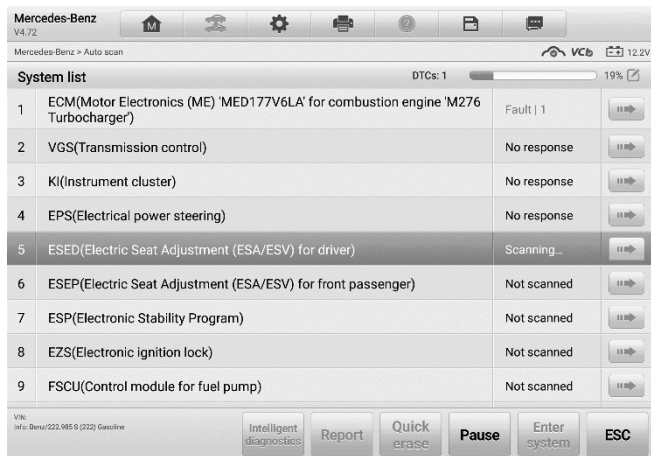
Figure 5-2 Fault Scan on System List Screen 2
