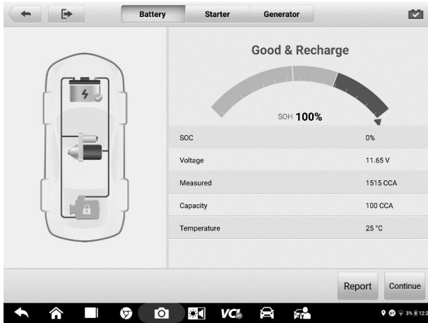
Figure 10-6 Battery Test Results Screen
